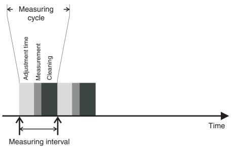
Fig. 3-6 Measuring cycle of the sensor
