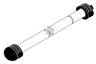
Fig. 3-3 Sensor with mounted shock protectors
