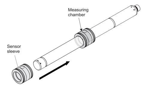
Fig. 4-4 Putting the sensor sleeve on the sensor
