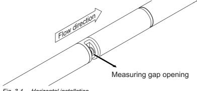
Fig. 3-1 Horizontal installation
