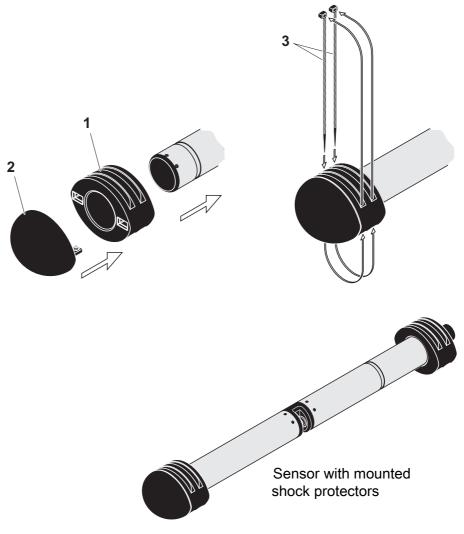
Fig. 3-4 Mounting the shock protectors
