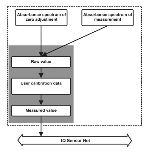
Fig. 4-1 Determination of measured values
