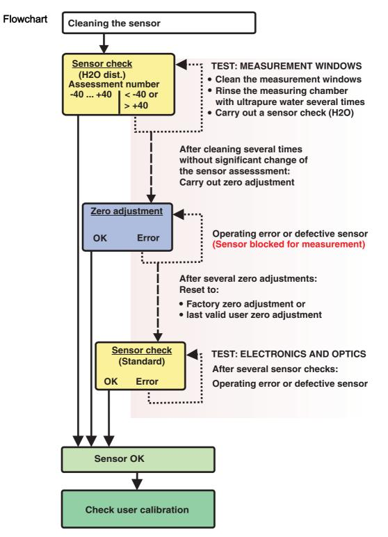
Fig. 4-3 Overview of Sensortest/Zero adjustment and user calibration.
