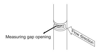
Fig. 3-2 Vertical installation
